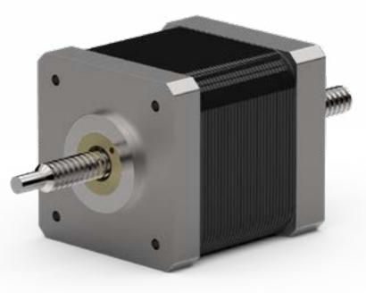
In a non-captive actuator linear actuator, the lead screw does not have an anti-rotation feature. Instead, external mechanical components separate from the motor are introduced into the design to keep the lead screw from rotating. As a result, the lead screw moves back and forth axially by restricting its rotation, which then drives the device it is attached to back and forth.
